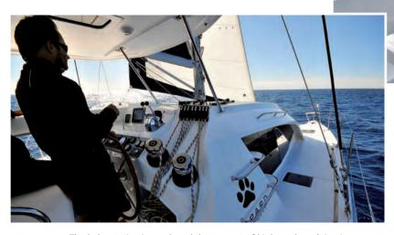
The helm station is good, and the amount of kit here doesn't impinge on sail handling, thanks to the assistance of the electric winch. Taking in a reef (with the continuous reefing lines) is easy, as is furling the genoa. Visibility is good, and the feel of the helm is direct thanks to the mechanical linkages.
