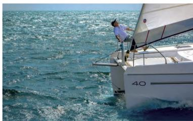
The Leopard 40 shows an overall balance which, thanks to the fineness of the hulls and good bridgedeck clearance (78cm), allows it to remain comfortable and perform well in a choppy sea, even upwind.
